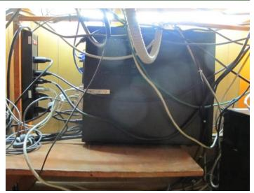
industrial computer with a solid-state drive. (Work still continues on making the remote station available to any Skyview member that wants to use it. I'm not happy with its current configuration. Stay tuned) To the left is an AC power srtip that's connected to UPS power. Along the top of the picture is the copper pipe that is used as the station ground bus. All major equipment is tied to this pipe.
