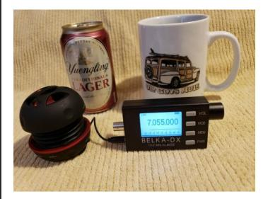
Coverage is continuous from 1.5 to 31 MHz. It has CW, USB, LSB, AM, and NFM modes With the minimal set of menu driven multi-function buttons, it takes a little longer to move around. But I setup memories to jump right to a ham band. Sensitivity and selectivity are both pretty good.
