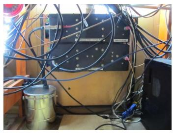
tion cabling is double shielded coax, either RG-400 or RG-214. This too is to help cut down on inter-station
