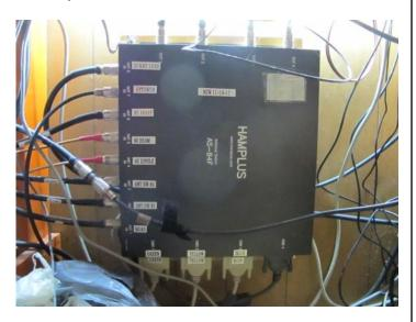
the left. Cabling from the four selector units connect on the bottom. The plastic bags you see on the bottom left hold oil filled dummy loads. I connect these up to antenna ports on the switch if one or two antennas are out of service. This way, if someone tries using an antenna that's not there, no damage is done.
