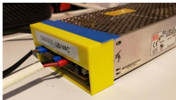
A Safety Cover for a repurposed Power Supply with 120VAC screw terminals at the end
