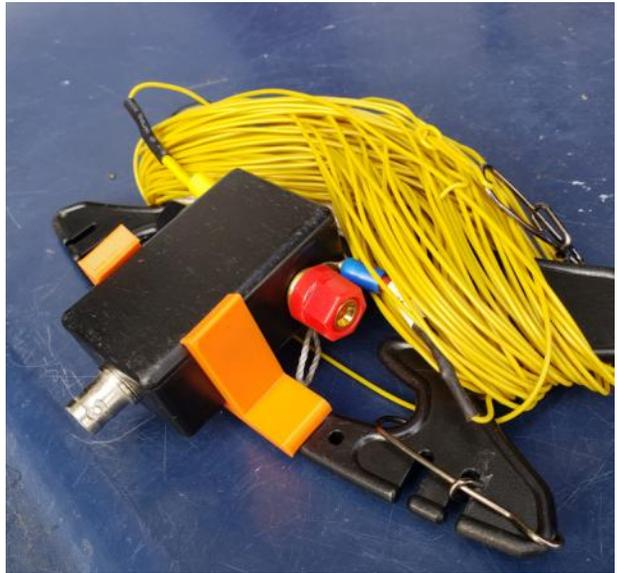
A simple, but effective Clamp to hold my SOTA Unun to my antenna winder while transporting it. It is glued to the winder. This went from "I Need Something" to Designed, Printed, and Glued to the Winder in about 2 hours
