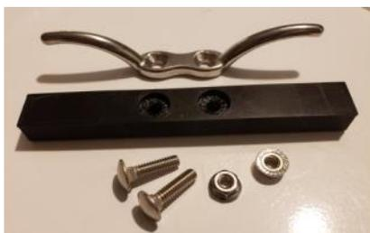
Adapters to allow adding Rope Cleats to my Push-Up Flagpole holding up my Dipole. (Cannot use screws to install Cleats with a Push-Up Flagpole.)
