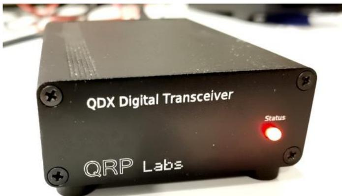
While designed mainly for WSJT-X modes, it can be used for any digital mode that only transmits a single tone at a time, such as RTTY. (There is an exception for CW/Morse as it is not designed to limit key clicks in that mode.) It has a Tayloe IQ receive detector and an internal sound card. So it only needs USB, power, and antenna connections.
