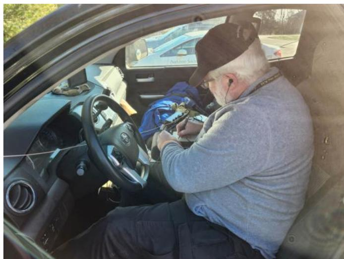
I operated an Elecraft KX2 using CW mode with a Tufteln 35 ft random wire antenna with 17 ft counterpoise suspended vertically from a tree branch. My radio and logging clipboard fit neatly on the console of my truck, with the antenna feedline running in through the door seal. I felt positively decadent operating from a seat with lumbar support instead of sitting on the ground.
