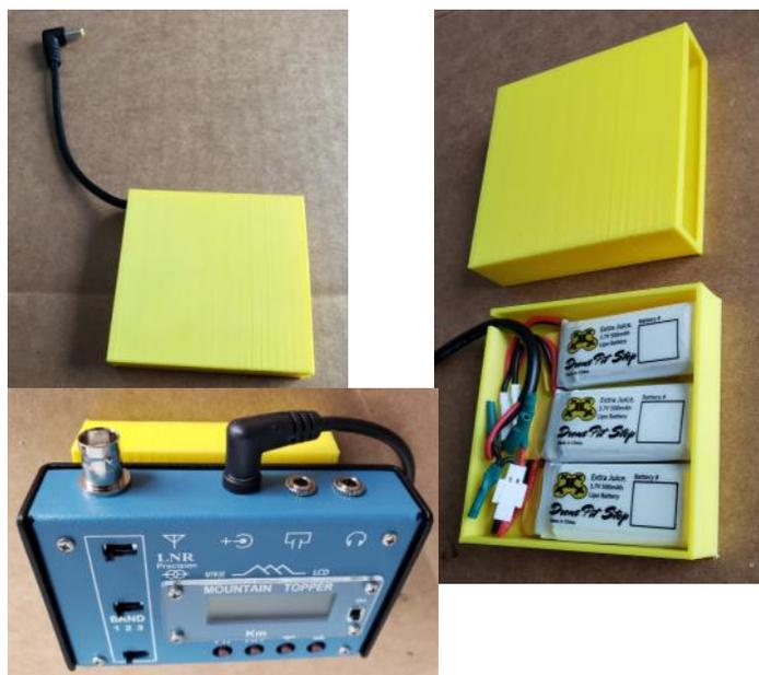
Another 'Matchbox' style Battery Case for an even a smaller battery pack that I will use with my MTR-3B transceiver. These battery cases attach to the MTR-3B with Velcro.
