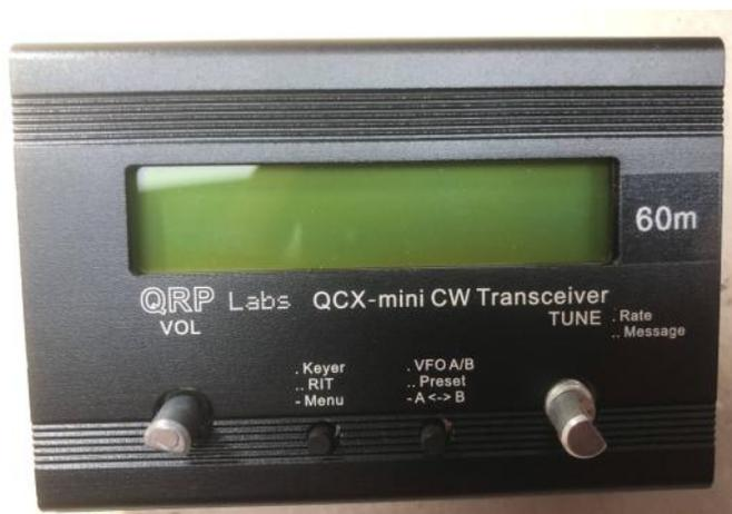
So, I decided to redo the kit for 80 meters instead. It seemed a rather simple change. Simply change a few low pass filter toroids and capacitors, rewind the band pass transformer, recalibrate and it's all
