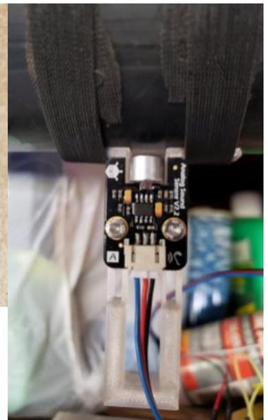
Another Mounting Bracket for a different sensor. This one allowed an adjustable positioning.
