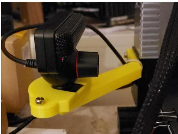
A Custom Bracket to hold a Camera that allows me to remotely watch my 3D Print Jobs. It works with a Raspberry Pi that sends the video output to my computer
