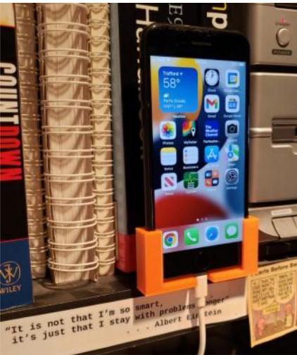
A Bracket to hold a Cell Phone on a bookshelf. This cell phone stays here all of the time—it replaced a landline. Previously it was held up with a piece of plywood with a couple nails driven in it to hold the phone upright. This bracket works much better
