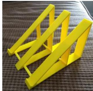
A stand to orient my Xiegu G90 at a convenient working angle on my desk. This is three separate printed sloped pieces, with two small printed struts. Super Glue holds it all together.
