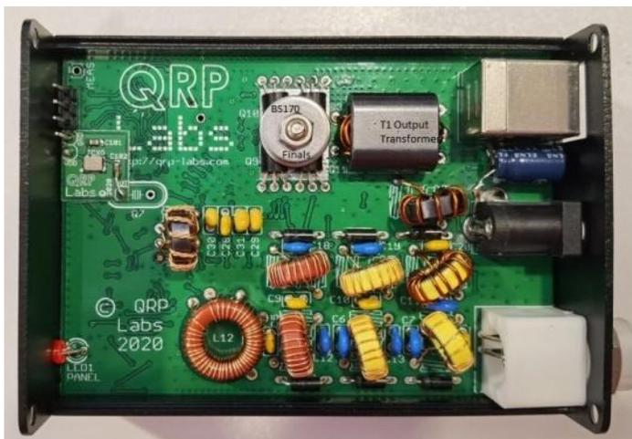
This seemed rather excessive to me, especially since the TO-92 transistor case does not conduct heat very well. The junction can take up to 150 C, but the hotter it is, the shorter its life is likely to be, especially if ambient temperature is high as well. In addition, the BS170's power dissipation is derated above 25 C.
