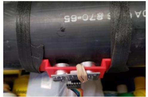
A Mounting Bracket for a sensor. I was chasing an intermittent water problem - needed to monitor the drain.
