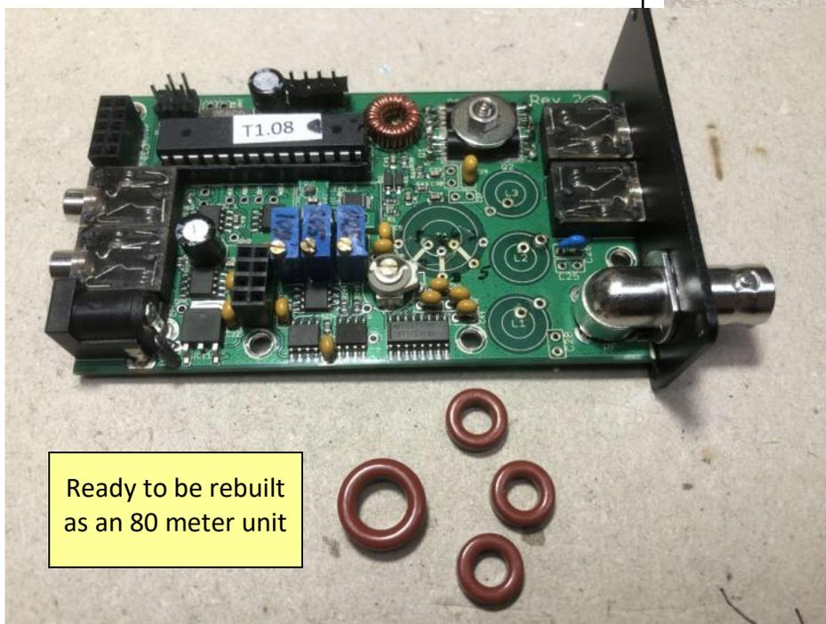
Calibration went well, but I had low power output of 3.2 watts. (Expected power out is 5 watts.) I found I had a little too much inductance on the LPF toroids, so I removed a few turns from each. Power then came up to about 3.5 watts.
