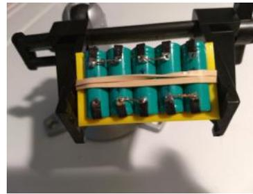
A temporary Fixture to hold five batteries in place while soldering the cell to cell jumper connections
