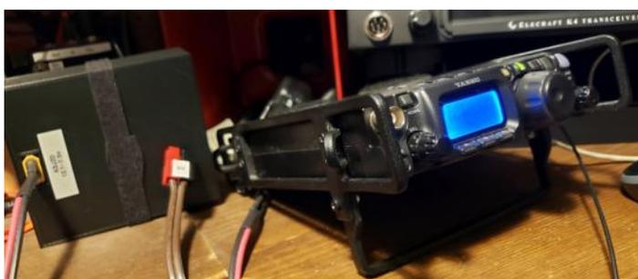
Case for a FT-817 External Battery. The purchased Battery Management Board uses three 3.1v 5000 mAH 21700 Lithium Ion Batteries. That's enough voltage to run the FT-817 at full power. But it came as a bare board that had traces on the back of the board. So I had to figure out how to design a case for it to allow taking it out to the field.
